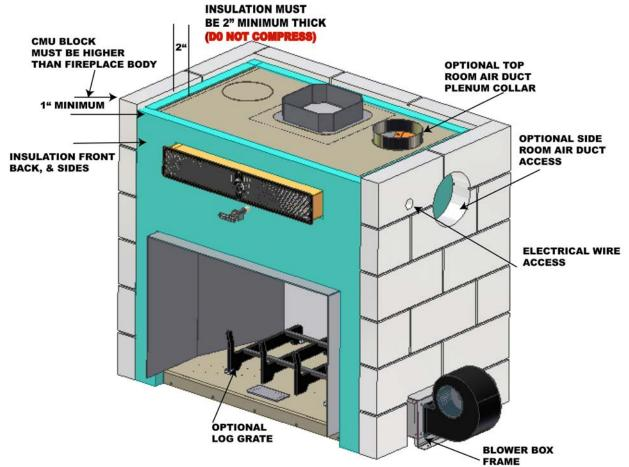
FIGURE 5: MASONRY WALL INSTALLATION
